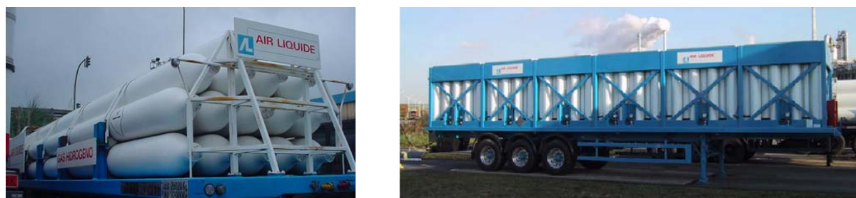
Figure 6: Two types of compressed gas hydrogen trailers operated by Air Liquide in Europe: tube trailer (left side) carrying 2000-3000 m 3 of hydrogen (depending on the numbers of tubes) and type II composite cylinder trailers (right side) carrying 6200 m 3 of H 2 (equivalent to 540 kg). Picture courtesy of Air Liquide.
