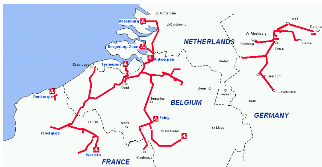
Figure 1: Hydrogen pipeline networks of Air Liquide in North-Europe (Benelux and France) and in the Ruhr area
